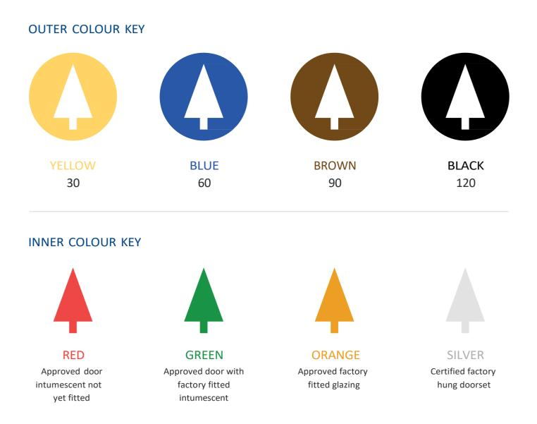
Plugs are fitted on the top edge of the door or the head of the frame.
